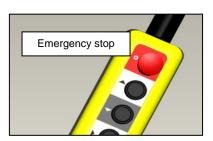
If the emergency stop is pressed, all functions will be immediately blocked and lifting, lowering, retracting or extending will stop. All functions can again be activated by turning the emergency stop to the right.
